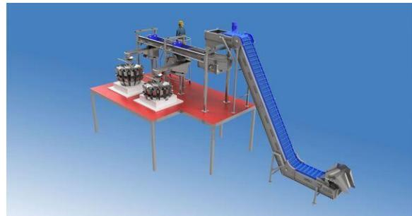
The production line, which will support Nutradia's drive to produce more healthy, non-fried snacks, includes Fabcon's modular horizontal motion and vibratory conveyors which can be extended to support further packaging stations at the central Belgium factory.
